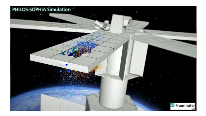
Snapshot of a simulated collision between a model of the LOFT (Large Observatory For X-ray Timing) satellite and a 12-unit CubeSat, moving with a relative velocity of 11 km/s and hitting at a 32 degree angle. LOFT is a candidate ESA Science mission competing for a launch opportunity in the early 2020s. At
