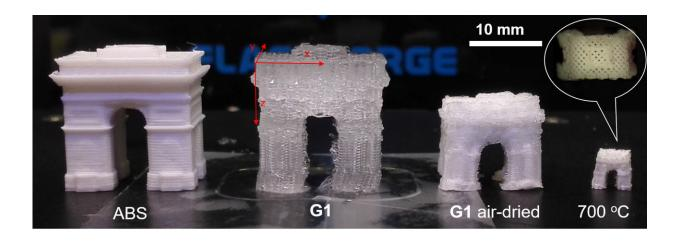
An example from the research shows how a 3-D-printed object composed of hydrogel (G1) can change size after printing. While this example serves to demonstrate the result, other objects can be used as filters or storage devices. Credit: Chenfeng Ke
