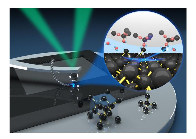
A single layer of silicon atoms (black) bind to the moving silica tip of a scanning probe microscope. Credit: Lei Chen/Southwest Jiaotong University
