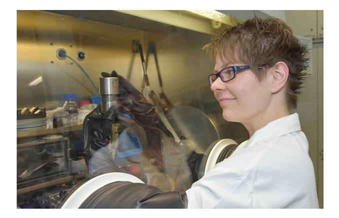
In the laboratory at the Faculty of Engineering, Hansen is constructing the first prototypes of silicon batteries, to test how many charge cycles they can last. There is no oxygen in this so-called "glove box", otherwise the lithium in the battery would oxidise. Credit: Julia Siekmann, Kiel University
