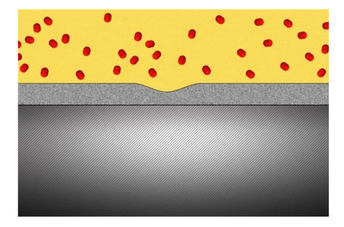
Researchers have found that a solid oxide protective coating for metals can, when applied in sufficiently thin layers, deform as if it were a liquid, filling any cracks and gaps as they form. Credit: Christine Daniloff/MIT
