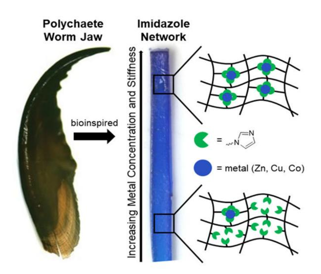
Scientists created a bioinspired gradient in mechanical properties. The range is achieved by programming the density of a special interaction between metal ions and electron-donating ligands. The left image is a polychaete worm jaw that uses
