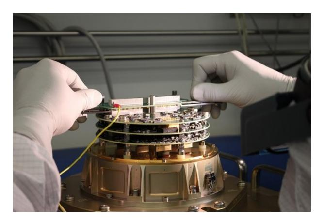
A set of flight camera electronics on one of the TESS cameras, developed by the MIT Kavli Institute for Astrophysics and Space Research (MKI), will transmit exoplanet data from the camera to a computer aboard the spacecraft that will process it before transmitting it back to scientists on Earth. Credit: MIT Kavli Institute
