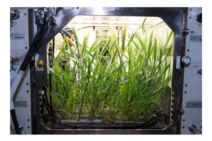
This image features green Dwarf Wheat within APH. The door of the facility has been removed to show the growth chamber within. Credit: NASA
