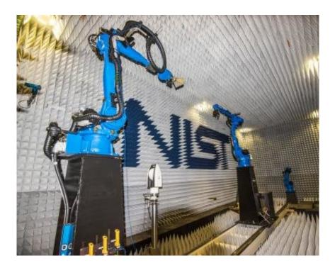
NIST's new Large Antenna Positioning System (LAPS) uses two robotic arms to measure and test antennas for applications such as advanced communications systems. Credit: Burrus/NIST
