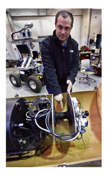
In this photo made on Wednesday, April 4, 2018, David Kohandash, a lead software technician in the robotics institute at Carnegie-Mellon University in Pittsburgh, points out the radiation sensors on the RadPiper robot designed to measure potentially hazardous radiation. The mechanism is intended to go through pipes at a former uranium plant being cleaned up in southern Ohio. (AP Photo/Keith Srakocic)
