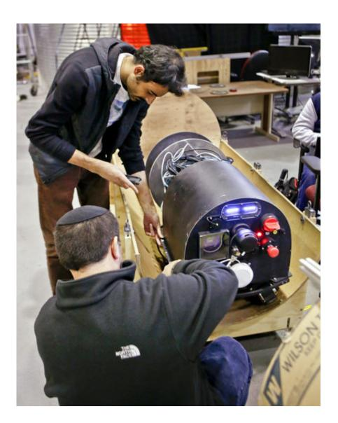
In this photo made on Wednesday, April 4, 2018, Mohammad Mousaei, top, and David Kohandash work on the RadPiper robot in the robotics institute at Carnegie-Mellon University in Pittsburgh. The mechanism is designed to measure potentially hazardous radiation is intended to go through pipes at a
