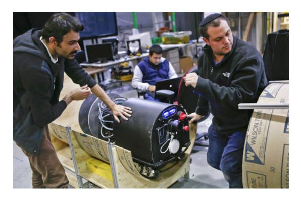
In this photo made on Wednesday, April 4, 2018, Nikhil Jog, center, works on a computer as Mohammad Mousaei, left, and David Kohandash, right, work on the RadPiper robot in the robotics institute at Carnegie-Mellon University in Pittsburgh. The mechanism is designed to measure potentially hazardous radiation is intended to go through pipes at a former uranium plant being cleaned up in southern Ohio. (AP Photo/Keith Srakocic)
