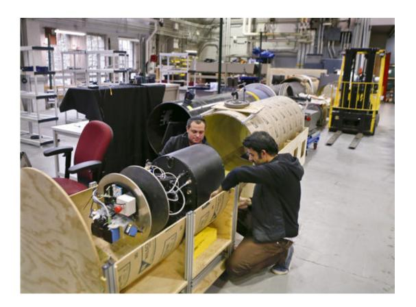
In this photo made on Wednesday, April 4, 2018, David Kohandash, left, and Mohammad Mousaei work on the RadPiper robot in the robotics institute at Carnegie-Mellon University in Pittsburgh. The mechanism is designed to measure potentially hazardous radiation is intended to go through pipes at a former uranium plant being cleaned up in southern Ohio. (AP Photo/Keith Srakocic)
