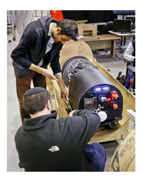
In this photo made on Wednesday, April 4, 2018, Mohammad Mousaei, top, and David Kohandash work on the RadPiper robot in the robotics institute at Carnegie-Mellon University in Pittsburgh. The mechanism is designed to measure potentially hazardous radiation is intended to go through pipes at a
