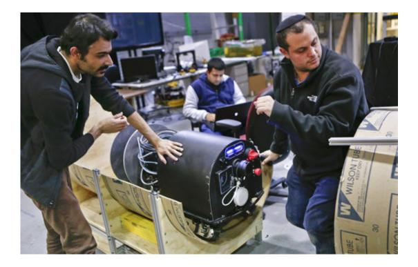
In this photo made on Wednesday, April 4, 2018, Nikhil Jog, center, works on a computer as Mohammad Mousaei, left, and David Kohandash, right, work on the RadPiper robot in the robotics institute at Carnegie-Mellon University in Pittsburgh. The mechanism is designed to measure potentially hazardous radiation is intended to go through pipes at a former uranium plant being cleaned up in southern Ohio. (AP Photo/Keith Srakocic)
