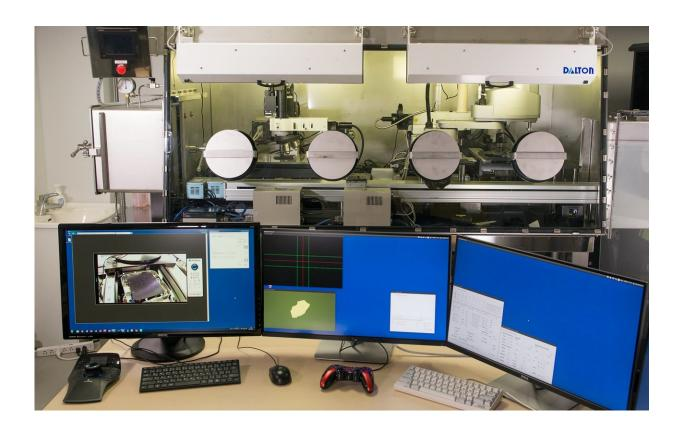
Robot developed for automated assembly of designer nanomaterials. Credit: University of Tokyo
