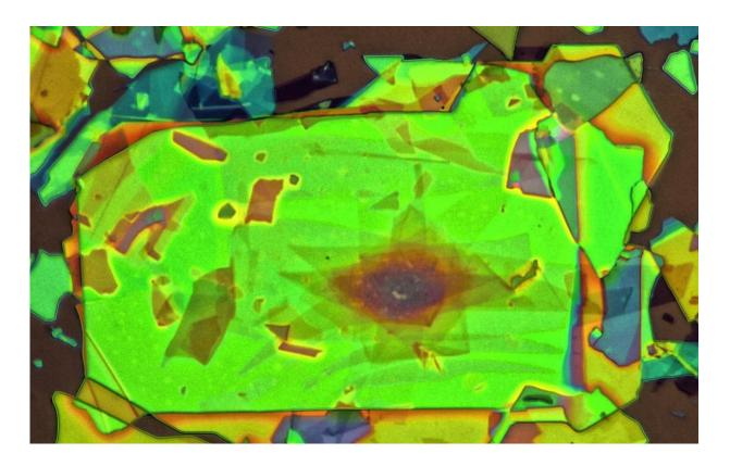
van der Waals heterostructures consisting of 29 alternating layers of graphene and hexagonal boron nitride. Credit: University of Tokyo
