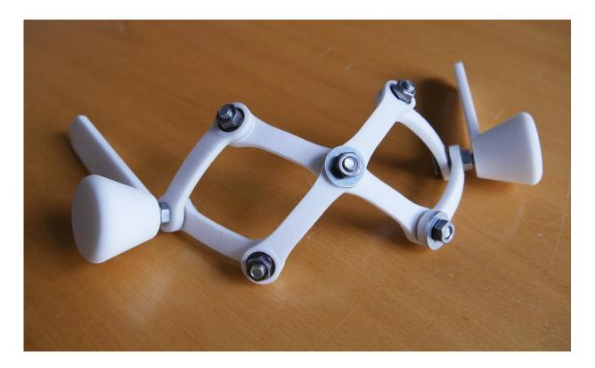
The CXD joint is the first joint in the world that can be pulled freely around a sphere. It provides freedom of movement to the shoulders or other of the body's ball-and-socket joints. Credit: Jakob Brodersen
