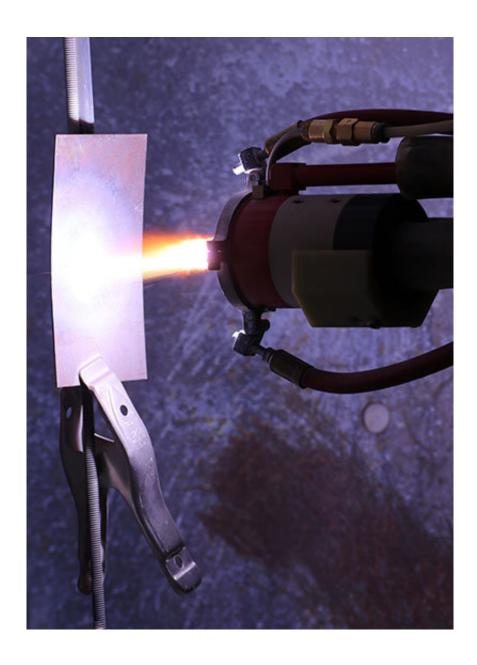
Plasma torch depositing recycled magnet material. Credit: Ames Laboratory
