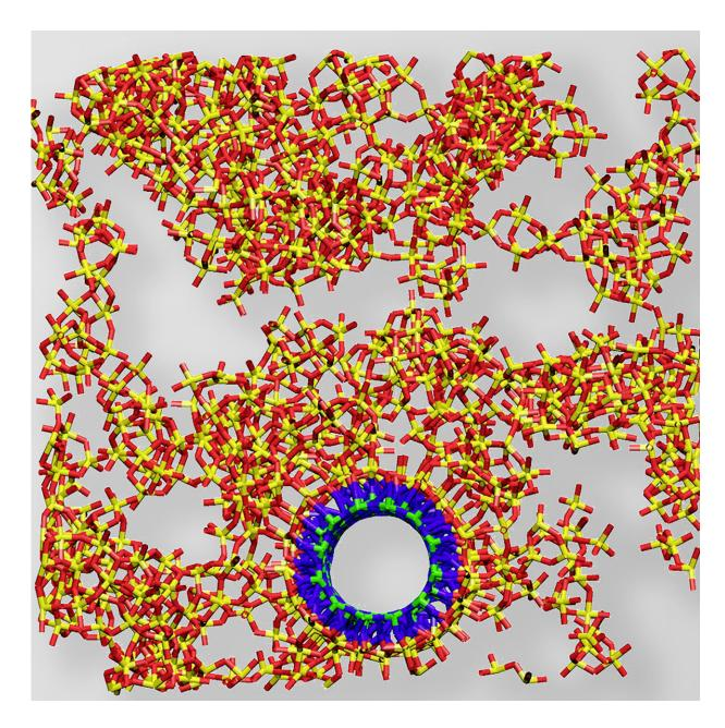
Boron nitride nanotubes in a silica matrix. Representation of reinforced nanomaterials with the Fraunhofer software. Credit: Fraunhofer SCAI
