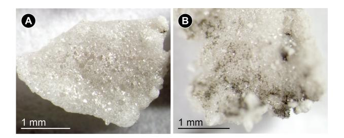
Samples of impact glasses created during an impact experiment. In impact experiments, these glasses capture surprisingly large amounts of water delivered by water-rich, asteroid-like impactors. Credit: Terik Daly
