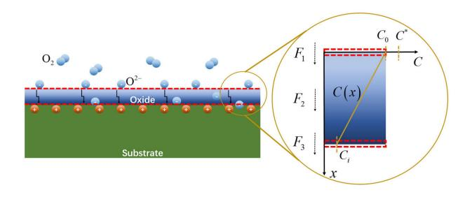
Schematic of an oxide film/substrate system and the oxidation process. In the first stage, the flux affects the diffusion and adsorption of oxygen from gas to the gas/oxide interface. Credit: Mengkun Yue
