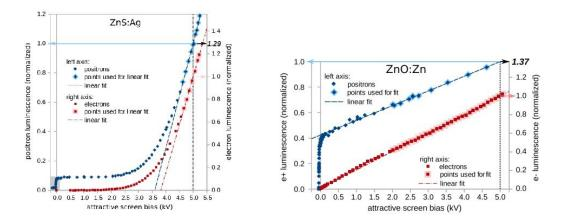
Differences between electron luminescence and positron luminescence for two different phosphors, ZnS:Ag and ZnO:Zn. Credit: Stenson et al. ©2018 American Physical Society
