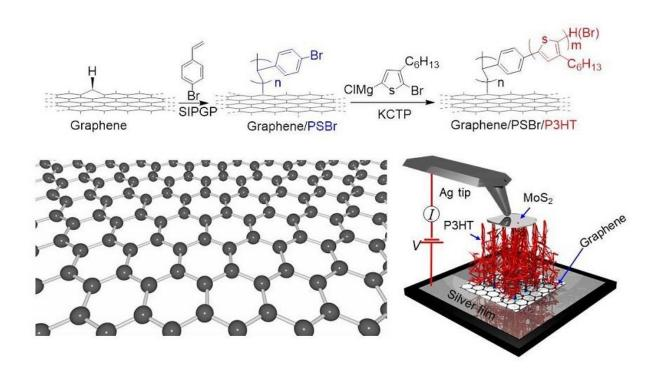
The scheme for obtaining a hybrid structure of 'graphene-polymer'. Credit: Tomsk Polytechnic University
