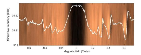
The color plot represents the current of electrons as the magnetic field and frequency of microwaves is varied. The white line highlights the strong dependence of the current on the direction of the magnetic field. Credit: OIST
