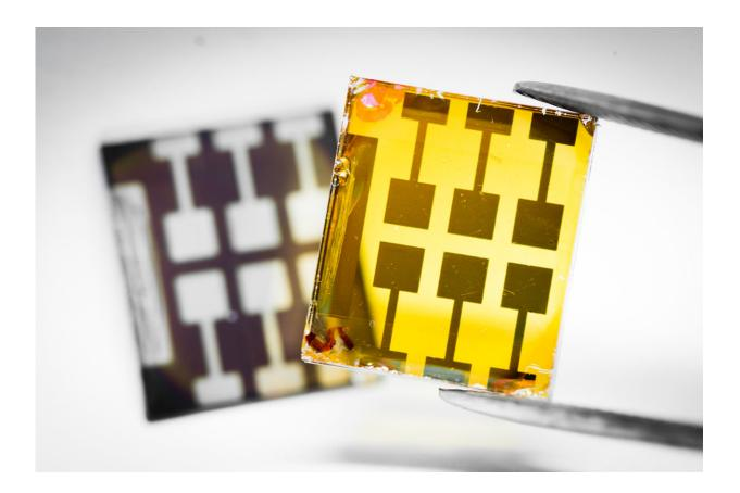
The lead-free double perovskite solar cells (yellow, in the front) compared with the lead-based device (dark, in the background). The next step is tune the color of the double perovskites into dark, so that they can absorb more light for efficient solar cells. Credit: Thor Balkhed
