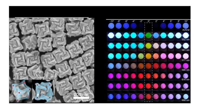
Electron microscope image of synthesized chiral gold nanoparticles (LEFT), where chiral components are highlighted in blue. Potential application in a color display as a three dimensional polarizer. (Right) Credit: Ki Tae Nam Research Group, Seoul National University
