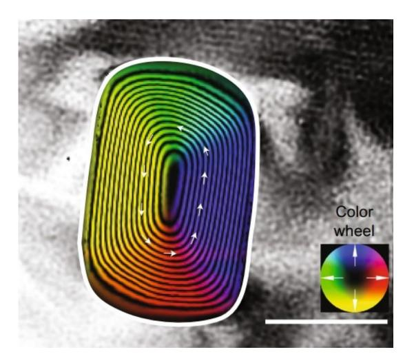
Magnetic induction map of a magnetically non-uniform kamacite grain (consisting mostly of iron), which is encased within a dusty olivine crystal in a meteorite. The arrows and the color wheel indicate the direction of magnetic induction. Scale bar: 200 nm. Credit: Shah et al. Published in *Nature Communications*
