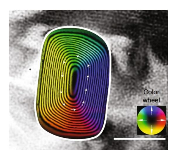
Magnetic induction map of a magnetically non-uniform kamacite grain (consisting mostly of iron), which is encased within a dusty olivine crystal in a meteorite. The arrows and the color wheel indicate the direction of magnetic induction. Scale bar: 200 nm. Credit: Shah et al. Published in *Nature Communications*
