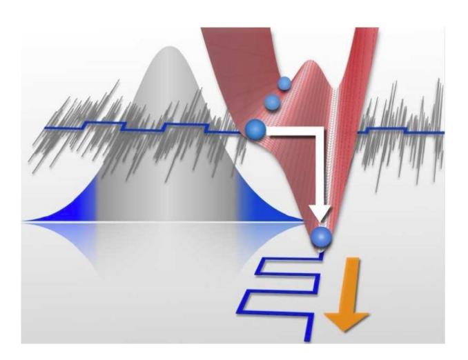
Conceptual illustration showing that sensitivity of the bistable system becomes high when Gaussian noise is imposed to a weak signal. Credit: Hokkaido University
