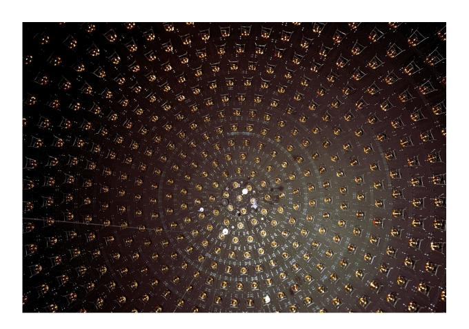
This interior view of the MiniBooNE detector tank shows the array of photodetectors used to pick up the light particles that are created when a neutrino interacts with a nucleus inside the tank. Credit: Reidar Hahn
