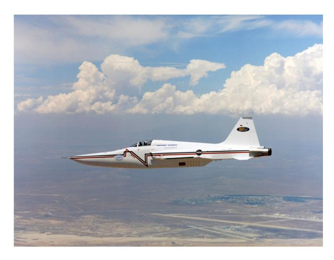
This modified Northrop F-5E jet was used during 2003 for NASA's Shaped Sonic Boom Demonstration program, a successful effort to show that an aircraft's shape can be used to reduce the intensity of the sonic booms it creates while flying supersonic. Credit: NASA
