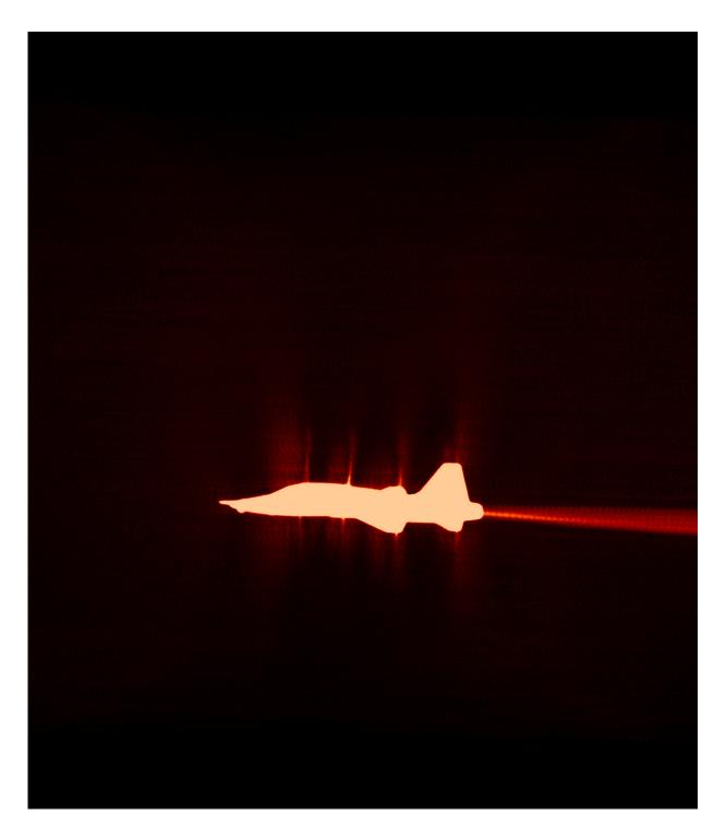
In this schlieren image, shockwaves are seen starting to form around this T-38. They propagate away from the aircraft and are heard on the ground as a sonic boom. NASA uses this imagery to study shockwaves and learn how to make sonic booms quieter. Credit: NASA
