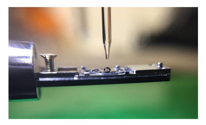
The new technology leverages a robotic system, designed by Gianneschi's group, which assembles chemicals needed for the experiment with high precision and reproducibility. Credit: The Gianneschi Group, Northwestern University
