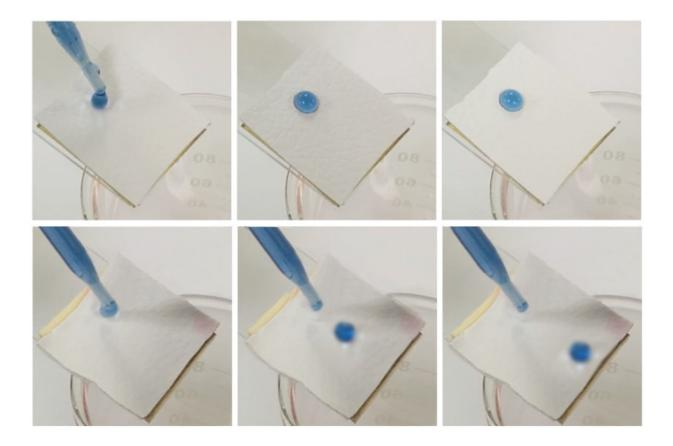
Researchers at The Ohio State University have invented a coating for synthetic leather that repels both water and oil. In these images, researchers place a drop of water on an untreated piece of synthetic leather (top, left to right) and a piece of treated synthetic leather (bottom, left to right). After treatment, the water rolls off. Credit: The Ohio State University.
