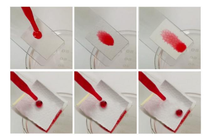
Researchers at The Ohio State University have invented a coating for synthetic leather that repels both water and oil. In these images, researchers place a drop of oil on an untreated piece of synthetic leather (top, left to right) and a piece of treated synthetic leather (bottom, left to right). After treatment, the oil rolls off. Credit: The Ohio State University.
