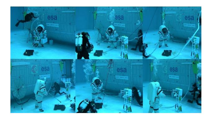
ESA's 10-m deep Neutral Buoyancy Facility at the European Astronaut Centre has been the site of the 'Moondive' study, using specially weighted spacesuits to simulate lunar gravity, which is just one sixth that of Earth. A database of items, tools and tasks that astronauts may have to handle on missions to the Moon formed the basis of Moondive activities, not just for training purposes but also for testing and validating new equipment and ways of doing things. Credit: ESA/COMEX
