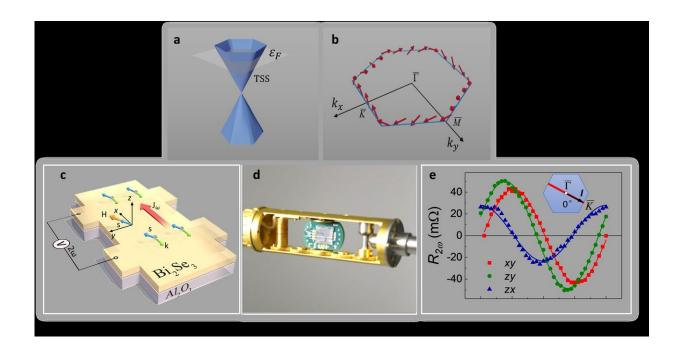
Figure: (a) Schematic diagram illustrating the Dirac cone of a topological insulator. (b) Spin-momentum locked surface state with hexagonal warping. (c,d) Hall bar device of topological insulator Bi2Se3 for harmonic resistance measurements. (e) Second harmonic resistance signal for the three scans of magnetic fields in xy, zy, and zx planes. Credit: National University of Singapore
