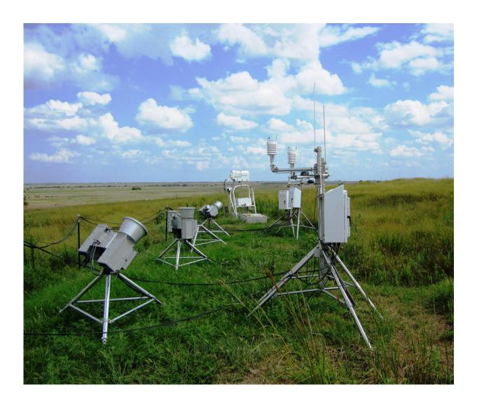
The scientists used radiometers, shown here, to isolate the signal of methane's greenhouse effect. Radiometers are among the many instruments at ARM's
