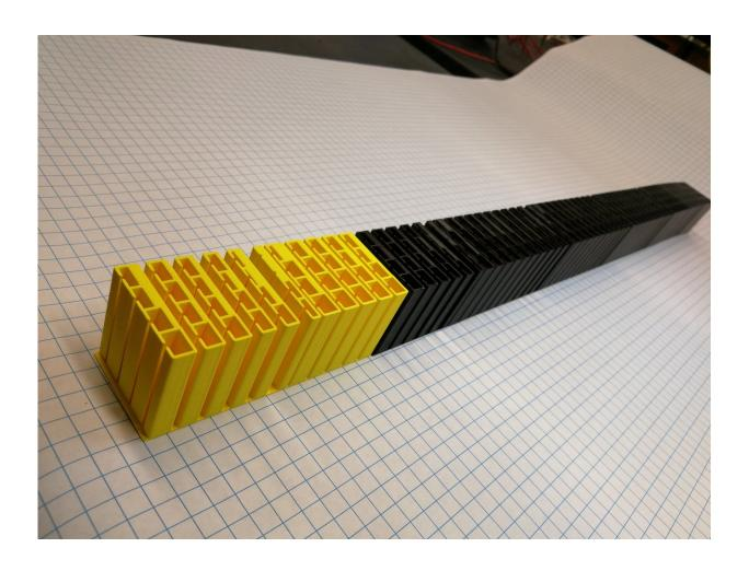
This metamaterial surface has been engineered to perfectly and simultaneously control the transmission and reflection of incoming sound waves. Credit: Junfei Li
