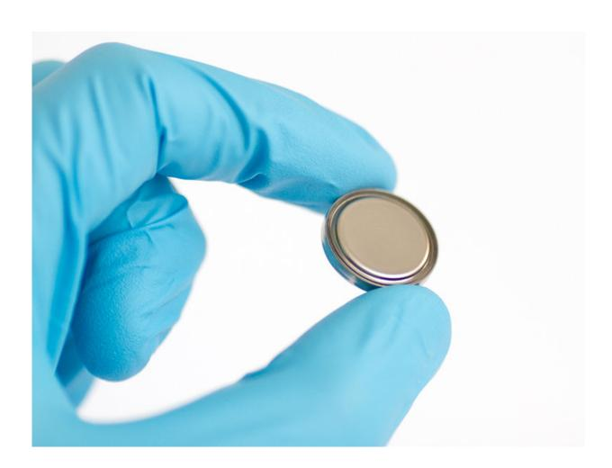
The researchers produced aluminum button cells in the laboratory. The battery case is made of stainless steel coated with titanium nitride on the inside to make it corrosion resistant. Credit: ETH Zurich / Kostiantyn Kravchyk
