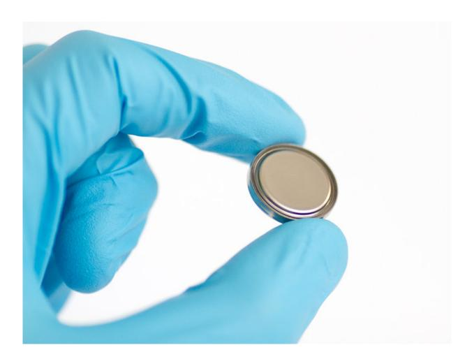
The researchers produced aluminum button cells in the laboratory. The battery case is made of stainless steel coated with titanium nitride on the inside to make it corrosion resistant. Credit: ETH Zurich / Kostiantyn Kravchyk
