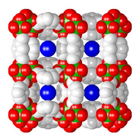
Different atoms (green = aluminium, red = oxygen, grey = carbon) together form the framework structure of CAU-10-H, which was developed at Kiel University. In the large pores, it can absorb and release water molecules (blue) highly efficiently. Credit: Dirk Lenzen
