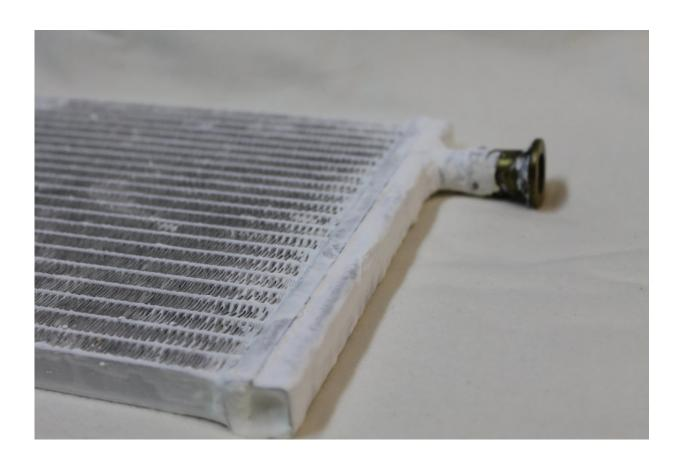
For their tests, they coated a conventional heat exchanger (as used in commercial refrigeration equipment) with the new material, in cooperation with colleagues from the Fraunhofer Institute for Solar Energy Systems. Credit: Dirk Lenzen
