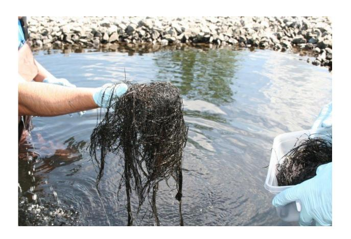
Biogenic manganese oxide-coated coir fiber collected from the coal mine drainage treatment system in Glasgow, Pennsylvania. Credit: Penn State
