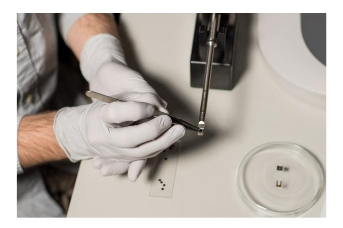
The research team create a tiny device that allows more of the microscope's electron beam to pass through liquid samples. Credit: Pacific Northwest National Laboratory
