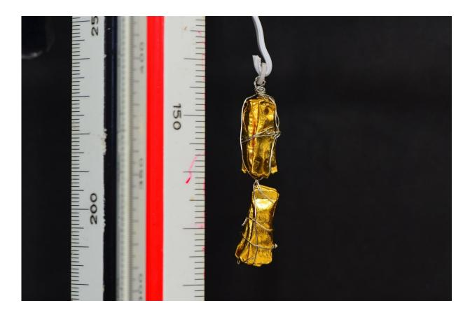
The samples were placed in small golden capsules -- with a melting point of 1,064°C -- and subjected to temperatures of 1,000-1,040°C and 1,000 times the atmospheric pressure of Earth. Credit: Lennart A. Fischer
