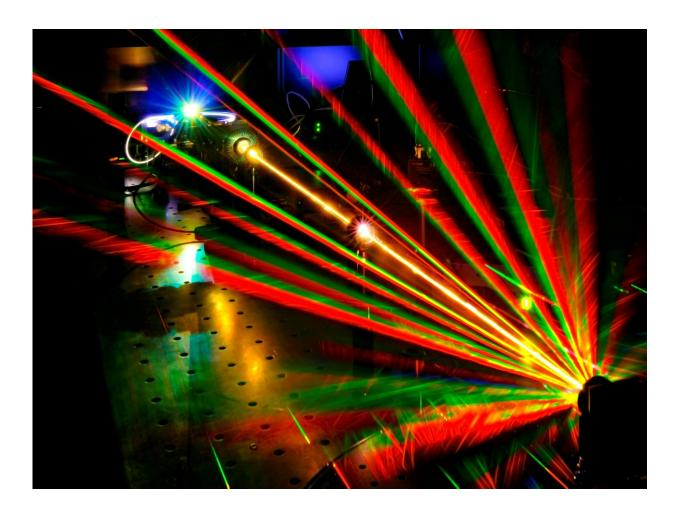
A twisted laser beam hits a nanoscopic U-shaped gold grating which further twists the beam in either a right or left-handed direction. This deflects the beam in many directions and further splits it into its constituent wavelengths across the color spectrum. Credit: Ventsislav Valev
