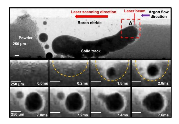
Using I12 and the LAMPR the complete process of track formation during 3D printing is revealed. A first complete track and details on the laser/gas flow are shown at the top. The first stages of the formation of this track are shown below for the first few milliseconds of track formation. Credit: Diamond Light Source
