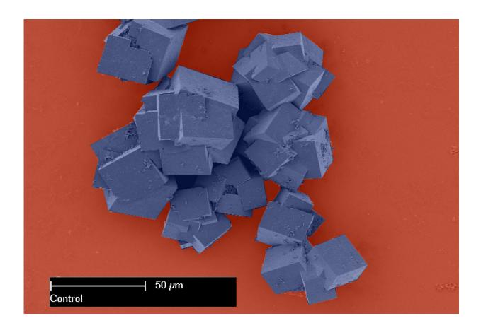
Metal-organic frameworks as seen under an electron microscope are made up of crystals that together shape multi-dimensional structures with vast surface areas. Credit: CSIRO/ Dr Paolo Falcaro, Dr Dario Buso, licensed under CC BY 3.0 (color changed)
