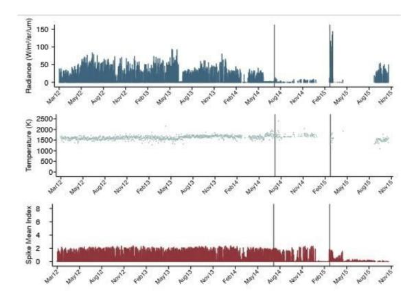
Dashboard for Ajil -- the dashboard shows data captured by remote sensing for Ajil oil field. The 'energy' activity at the field reflects production before IS took over (July 2014) after which production plummets; the field is taken back by government forces and the March 2015 spike in activity corresponds to IS fighters setting fire to the field; activity resumes in September 2015. Credit: Elsevier, Energy Research & Social Science (ERSS)
