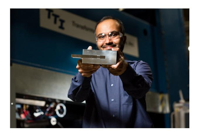
Friction Stir Dovetailing is a process that joins thick plates of aluminum to steel. The new process will be used to make lighter-weight military vehicles that are more agile and fuel efficient. Credit: PNNL
