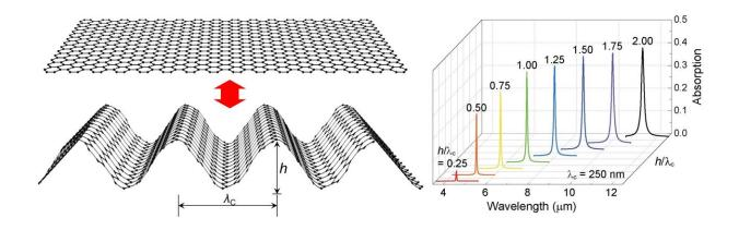
Mechanically tunable light absorption wavelength with wrinkled graphene structures. A schematic illustration of the uniaxially wrinkled graphene structure (left panel) showing a reversible mechanical change of the wrinkled structure. Optical absorption spectra (right panel) for the wrinkled graphene structures with various aspect ratio of wrinkle height (h) to wavelength ( $\lambda c$ ) Credit: University of Illinois College of Engineering
