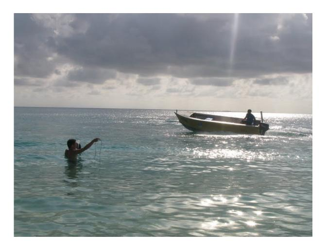
Researchers use a hydrophone to record and measure noise from a passing motorboat. Credit: Maud Ferrari
