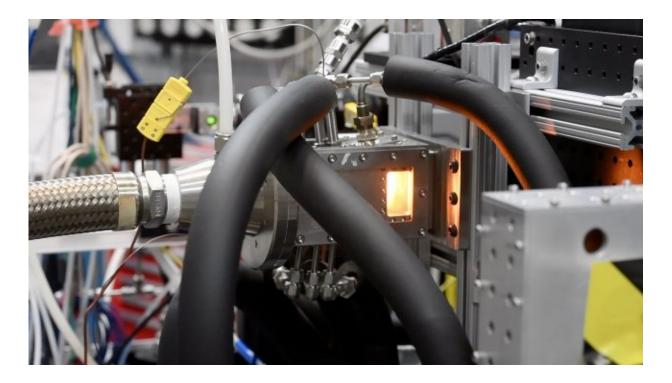
Team members from the U.S. Army Research Laboratory's Center for Unmanned Aircraft Systems Propulsion conduct an using powerful X-rays to see inside a gas turbine combustor during ignition. Researcher hope to use the data to optimize engine efficiency. Credit: U.S. Army photo by David McNally
