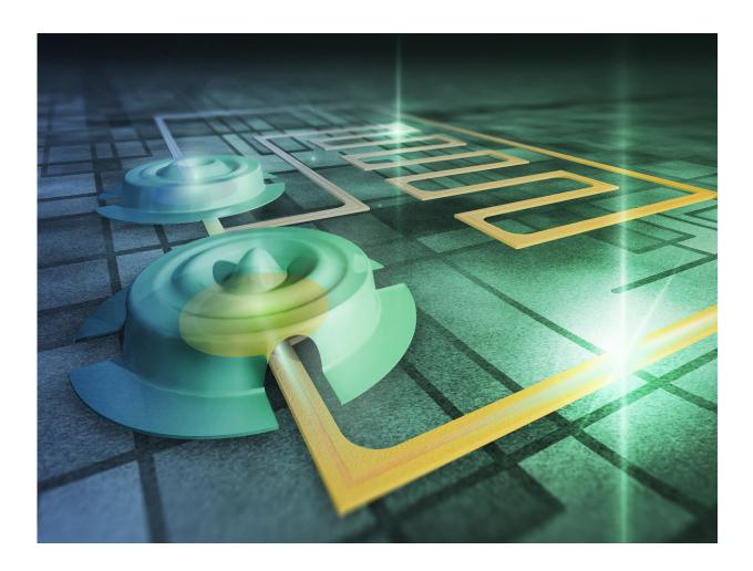
Illustration of the 15-micrometre-wide drumheads prepared on silicon chips used in the experiment. The drumheads vibrate at a high ultrasound frequency, and the peculiar quantum state predicted by Einstein was created from the vibrations. Credit: Aalto University/Petja Hyttinen & Olli Hanhirova, ARKH Architects.
