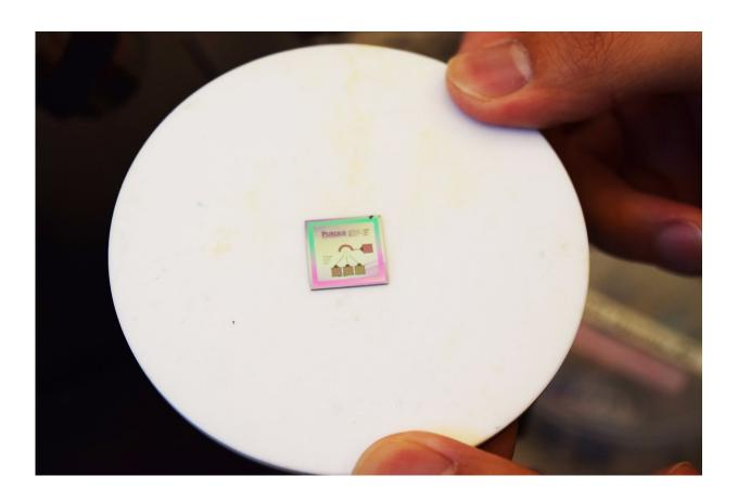
This small chip holds a 2-D electrode with a shape that can better stimulate small targets in the body over time. Credit: Purdue University image/Kayla Wiles
