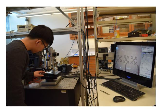
The fractal electrode shape, as seen from under a microscope, outperforms conventional circular or rectangular electrode shapes. Credit: Purdue University image/Kayla Wiles
