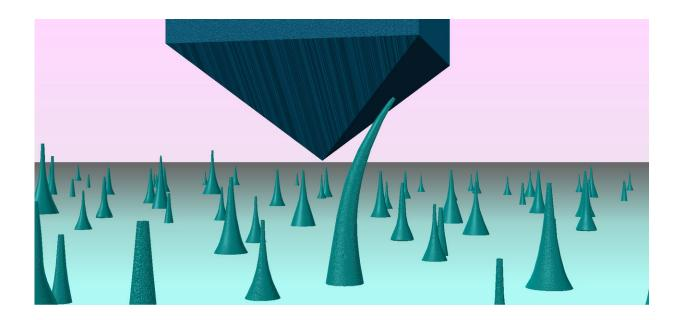
Schematic drawing of a diamond nanoneedle being bent by the side surface of a diamond tip, showing ultralarge elastic deformation. Credit: Yang Lu, Amit Banerjee, Daniel Bernoulli, Hongti Zhang, Ming Dao, Subra Suresh
