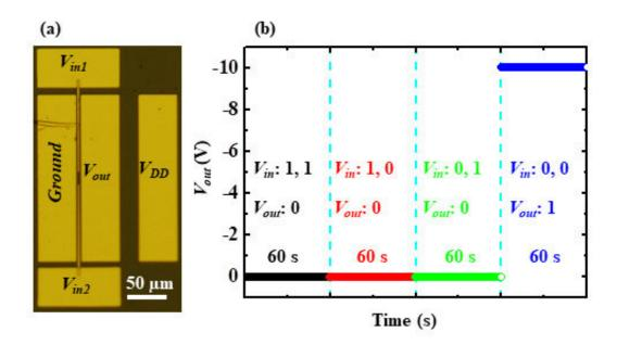
The view of the H-diamond MOSFET NOR logic circuit from above (left), and the operation of the NOR logic circuits, showing that the circuit only produces voltage when both inputs are at zero. Credit: Liu et al.
