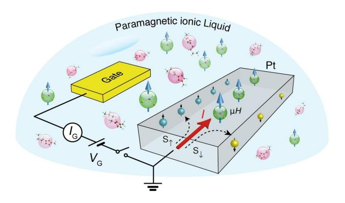
Schematic of Platinum transistor with paramagnetic ionic liquid gate. Credit: L. Liang
