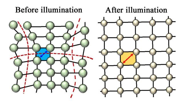
Constant illumination was found to relax the lattice of a perovskite-like material, making it more efficient at collecting sunlight and converting it to energy. The stable material was tested for solar cell use by scientists at Rice University and Los Alamos National Laboratory. Credit: Light to Energy Team/Los Alamos National Laboratory
